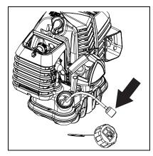
Note: Federal EPA regulations require all model year 2012 and later gasoline powered engines produced for sale in the United States to be equipped with a special low permeation fuel supply hose between the carburetor and fuel tank. When servicing model year 2012 and later equipment, only fuel supply hoses certified by EPA can be used to replace the original equipment supply hose. Fines up to \$37,500 may be enforced for using an un-certified replacement part.
