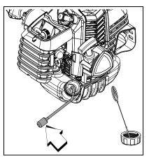
c. When the inside of the fuel tank is dirty, rinse the tank out with gasoline to clean it.
