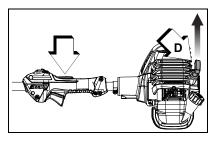
trigger and allow unit to warm up at idle for several minutes.
