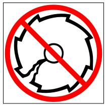
When sharpening a blade, always remove the same amount of materials from each tooth to maintain balance.
